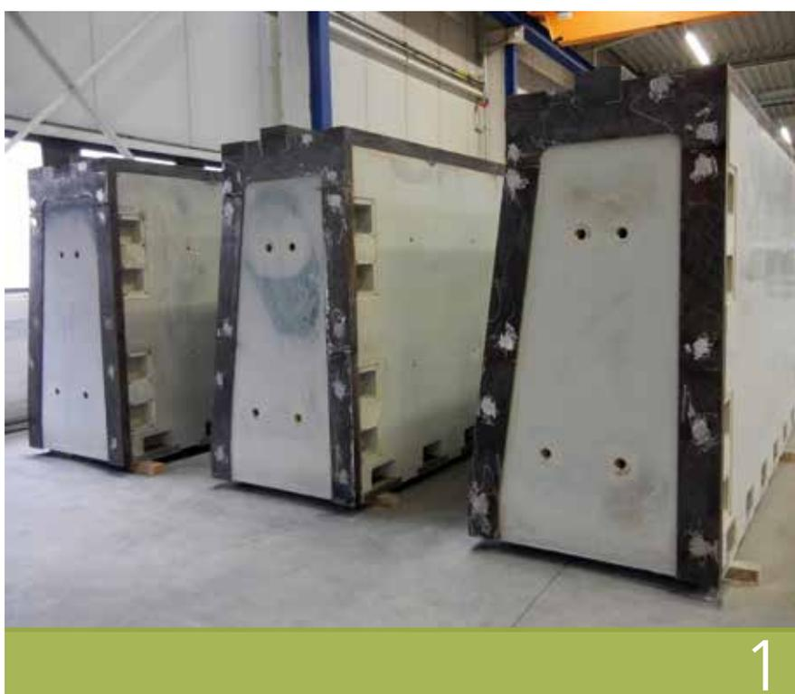
1. I SINGOLI ELEMENTI DELLA FRESATRICE PESANO 18 T (CIRCA 7,5 T DI NANODUR COMPOUND 5941 L'UNO) MILLING MACHINE'S INDIVIDUAL ELEMENTS WEIGHING 18 TONS (APPROXIMATELY 7.5 TONS OF NANODUR COMPOUND 5941 EACH)
